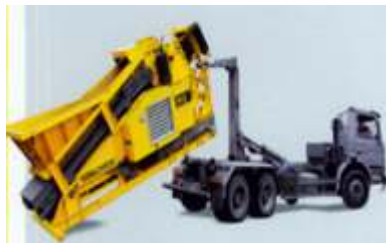
Fig. 6.12 a and 6.12 b Rubble Master with hook lift lorry
