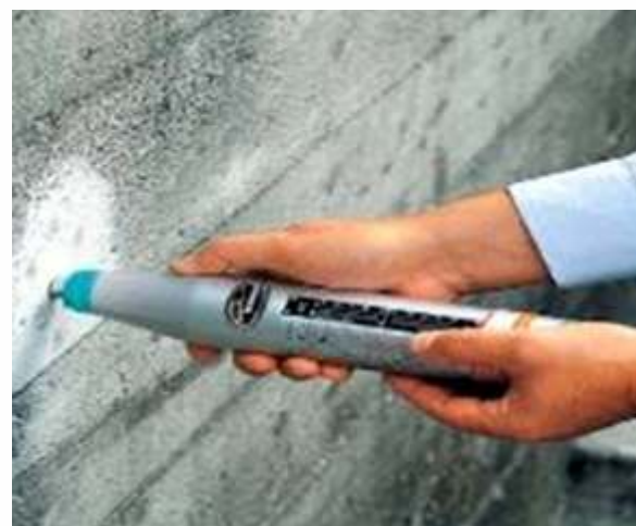
Fig. 2.2 Non-destructive testing (Rebound Hammer Test)
