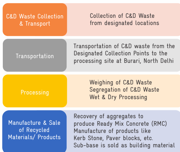
Fig. 1 Process flow of C&D waste collection, processing and recycling at Burari plant
