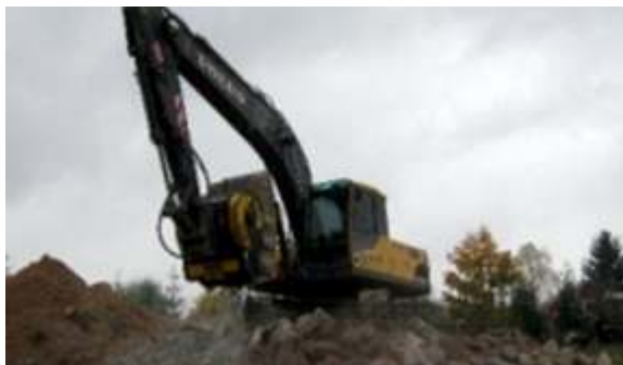
Fig. 5.38 Bucket Crusher for recycling
