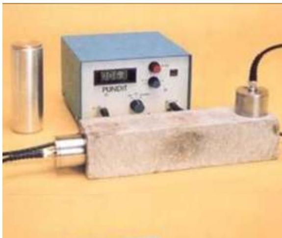
Fig. 2.4 Pulse velocity test
