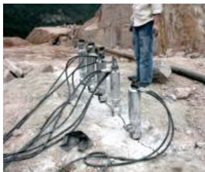
Fig. 5.8 Hydraulic Rock Splitter
